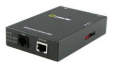
When you need to extend Ethernet services beyond the general IEEE 802.3 limits of 328ft / 100m, and new fiber cabling is cost prohibitive, **Ethernet Extenders** are the perfect solution. Perle Ethernet Extenders **transparently extend** up to four 10/100/1000 **Ethernet connections across copper wiring**. Use **single twisted pair** ( CAT5/6/7 ) **or any existing copper wiring** previously used in alarm circuits, E1/T1 circuits, RS-232, RS-422, RS-485, CCTV and CATV applications.
